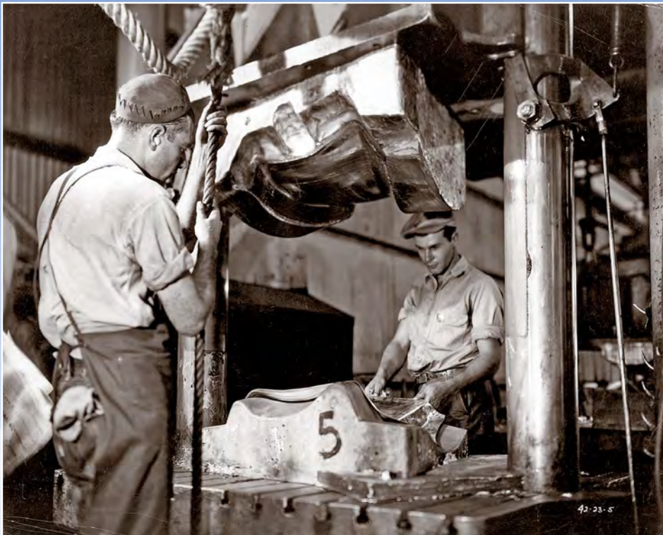
Factory workers used Rohr’s “drop hammer” machine to produce thinner and lighter metal for airplanes. The machine had a dramatic effect on the aircraft industry.
