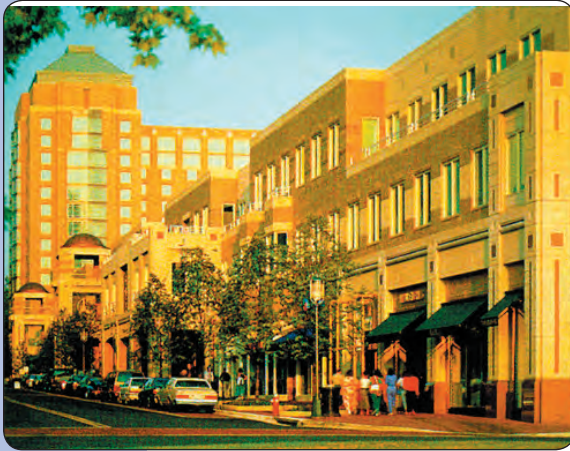
Buildings should form a continuous streetwall while upper floors step back Fig. 7.101
