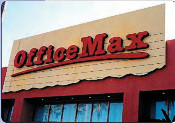
Oversized signs that project over the roof area are not allowed
