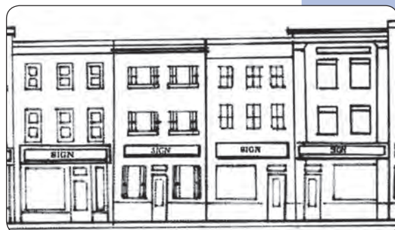
Wall signs of consistent size and placement establish facade rhythm
