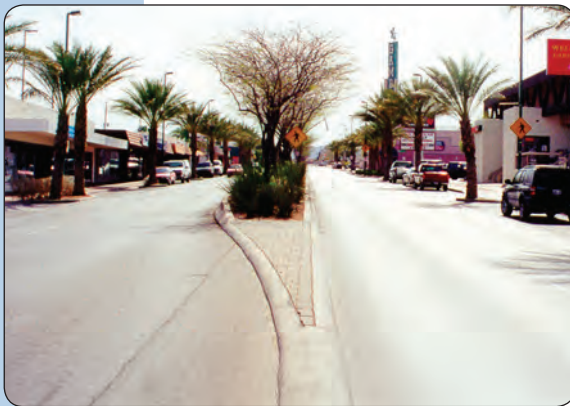
Medians with tapered ends should be enhanced with special paving
