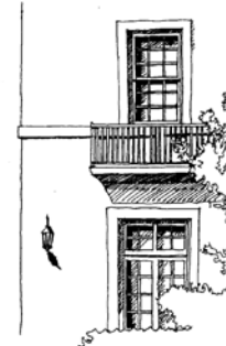
Aligned Window and Door Units with Casing, Metal Rail, Banding
