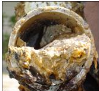
Prevent clogging of pipes. Don't pour Fats, Oils, or Grease down your drain.
