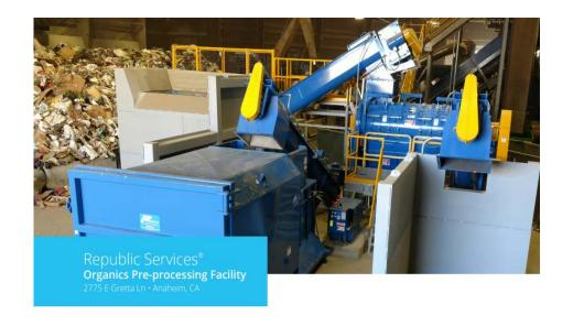
The MEGA THOR Turbo Separator effectively separates contamination from the food waste stream (SSO - Source Separated Organics).
