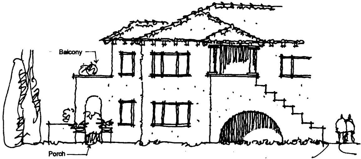
2-story stair element incorporating exterior stairs into building architecture.
