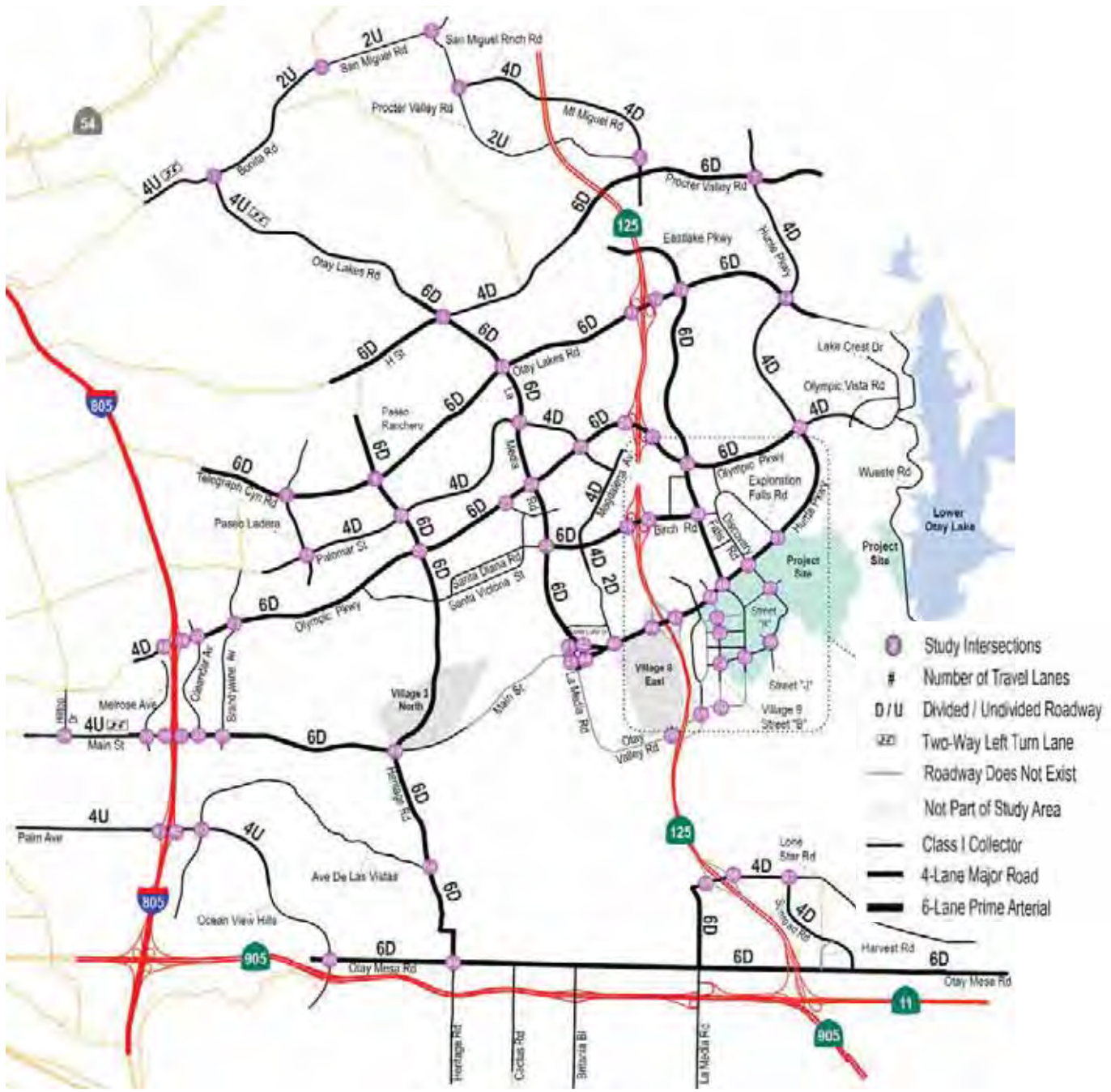
EXHIBIT 4.1.4: TRAFFIC IMPACT ANALYSIS PROJECT AREA – 2025 CONDITIONS
