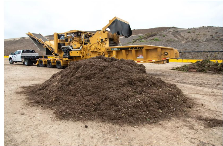
At the Olay Compost Facility, organic waste goes through a grinder that produces a fine mulch which is then covered, watered, and pumped with oxygen to speed up decomposition. (Jarrod Valliere / The San Diego Union-Tribune)
