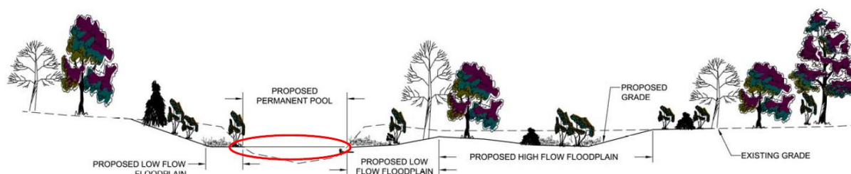
Figure 3. A cross-section of Stream Rehabilitation designed to maximize floodplain connection via overbank flooding
