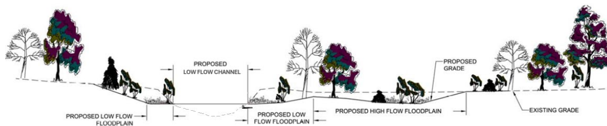
Figure 1. Example of Stream Rehabilitation with increased access to floodplain. This example would provide credits from the increased runoff retention in the proposed floodplain areas as well as increased biofiltration and ecological condition.
