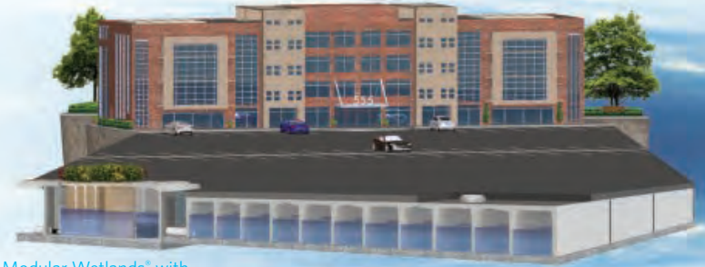
Modular Wetlands® with Box Culvert Prestorage
