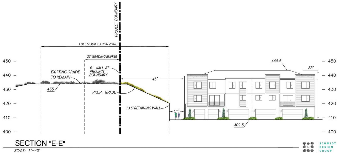
Exhibit 29: South Perimeter Condition @ R-6 (Cross Section E-E)
