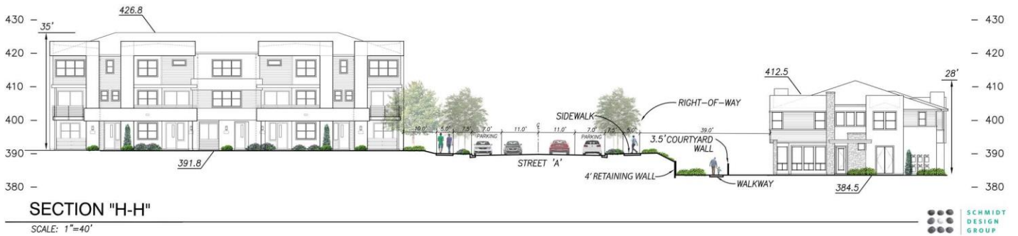
Exhibit 28: Internal Condition @ R-1 & R-4 (Cross Section H-H)
